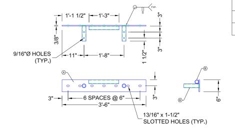
FABRICATE FROM ASTM A-36 STEEL. HOT DIP GALVANIZE AFTER FABRICATION IN COMPLIANCE WITH ASTM A-123-08. STAMP OR TAG PART I.D. ON EACH WELDMENT.
